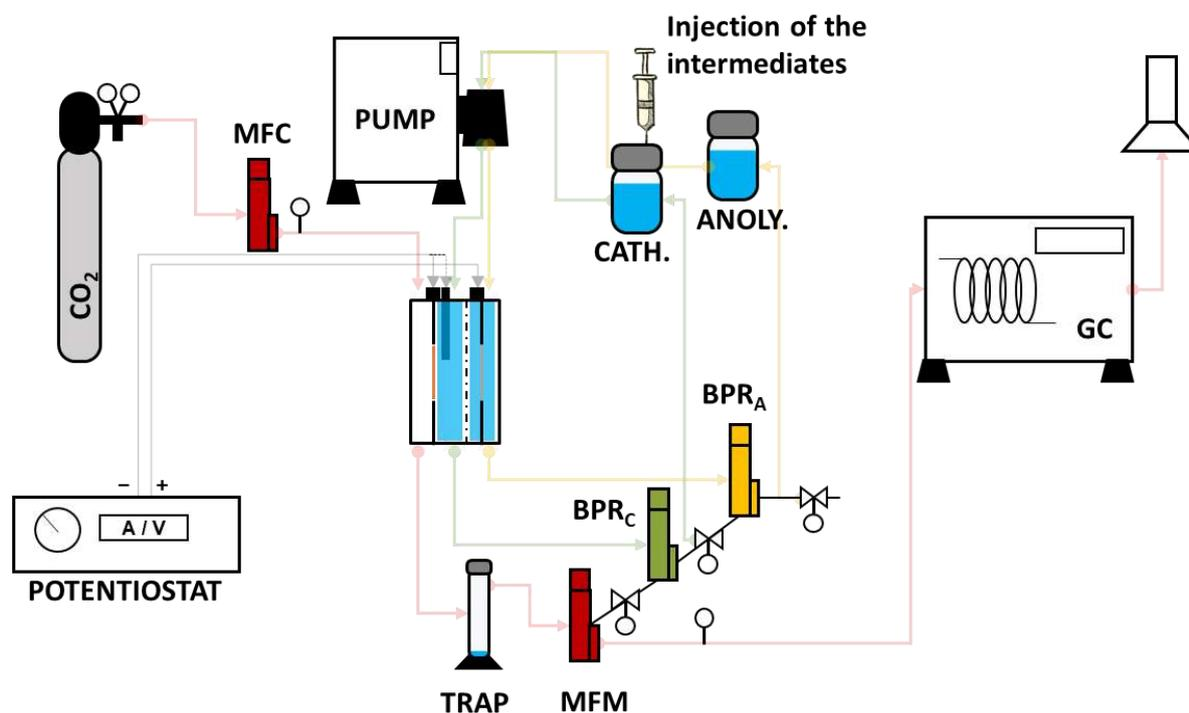
Figure 3: Experimental set-up used for the electrochemical CO<sub>2</sub> reduction reaction. MFC and MFM are for the mass flow controller and measurement, BPR<sub>C</sub> and BPR<sub>A</sub> are the back-pressure regulators for catholyte and anolyte compartments. The intermediates were injected with a volumetric syringe at the catholyte beaker.
