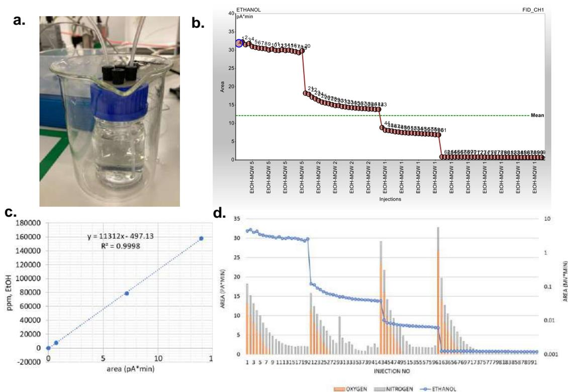
Figure 4: **a)** 100 mL solution of ethanol and MQ-water purged with He (not to interfere with N<sub>2</sub> or O<sub>2</sub> or to produce any other signal in the GC), **b)** Ethanol peak areas of the 92 GC injections **c)** Calibration plots for ppms of ethanol inside MQ-water vs. the GC-peak area **d)** Ethanol peak area in left-y axis and N<sub>2</sub> & O<sub>2</sub> area on the right-axis.
