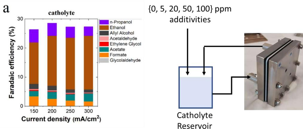
Figure 2: Overview of the minor liquid products reported by Ma et al. [4] during ECO2R on a copper catalyst at elevated current densities and a representation of the cell and simplified experiments performed within the deliverable.
