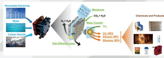
SELECTCO2 will develop enhanced electrolysis devices enabling CO<sub>2</sub> to be converted into high value chemicals. Specifically, it will improve selectivity, efficiency and durability of electrochemical CO<sub>2</sub> conversion into either carbon monoxide, ethanol or ethylene.
